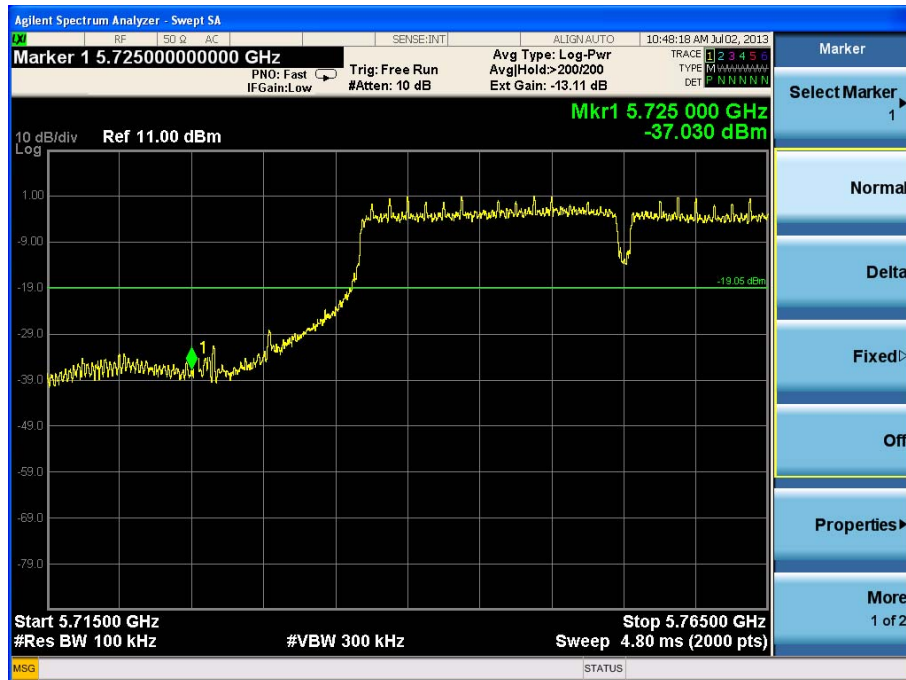
Figure 4.7.2 The Worst Out-of-Band Emissions Near Band Edge for 40MHz Carriers, 802.11n (40MHz-2Tx-1S) Carrier at Channel 151/5755MHz, 18dBm Setting (Both Medium Gain and High Gain Antenna), OFDM/CDD, MCS0, Port 1.
