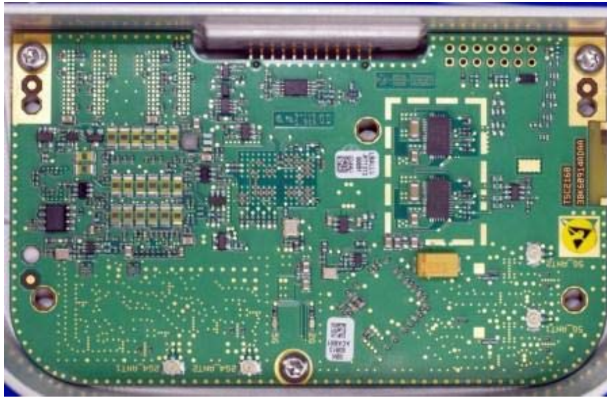
Internal View of MCO Wi-Fi AP Module with Antennas Removed
