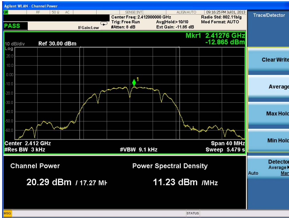
Figure 4.6.1 The PPSD Measured for 802.11b (20MHz-1Tx) Carrier at Channel 2412MHz, 21dBm (Medium Gain Antenna), DSSS, 1 Mbps, Port 2 (Total PPSD = -12.87dBm+3dB = -9.87dBm).
