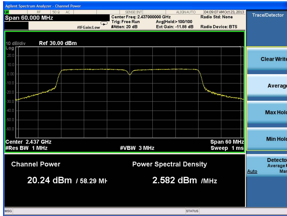
Figure 4.5.3 The Mean Output Power Measured for 802.11n (40MHz-2Tx-1S) Carrier at Channel 2437MHz, 20dBm (High Gain Antenna), OFDM/CDD, MCS0, Port 1.
