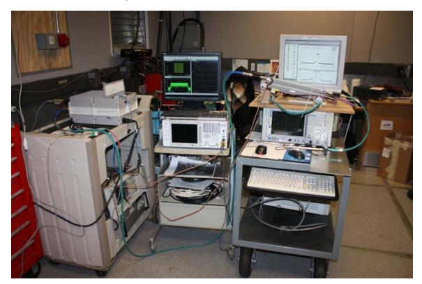
**TEST:** Measurement of Radiated Spurious Emissions
