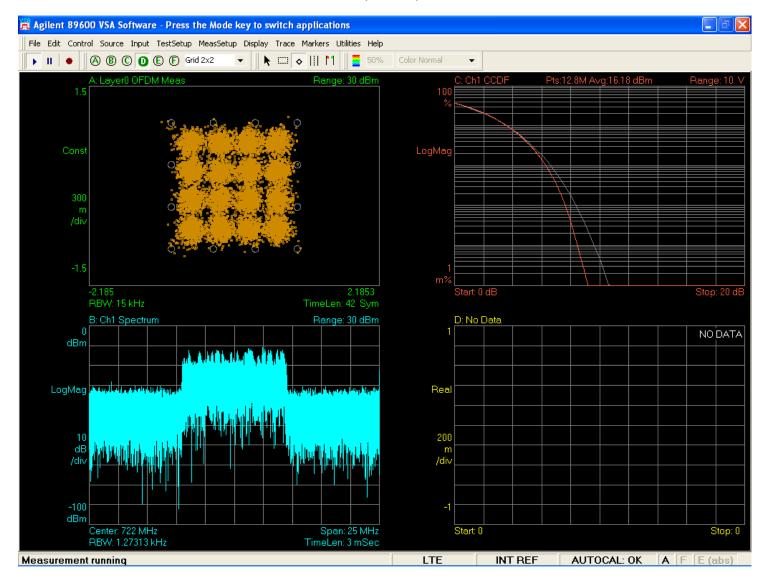
LTE 64QAM Tx1 722 MHz, 40W (46 dBm), 10 MHz BW
