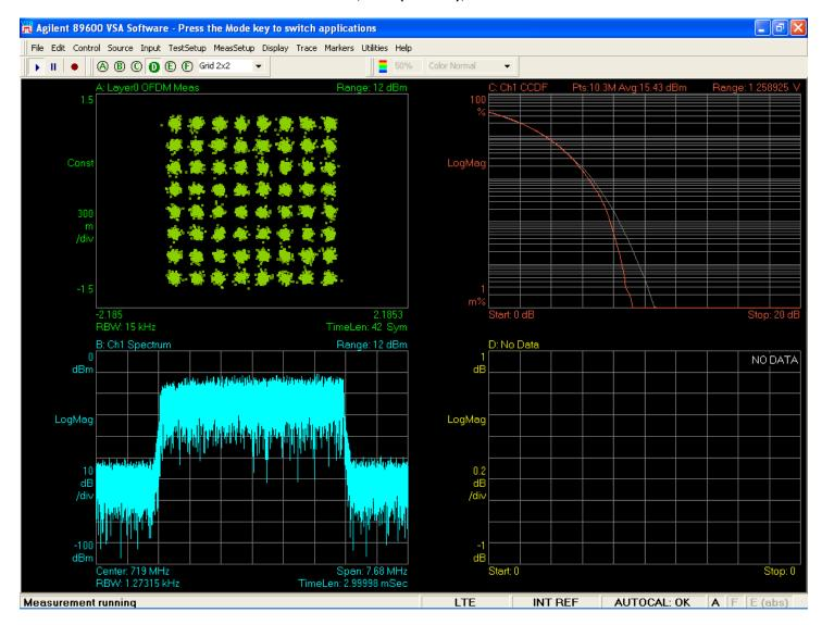
LTE QPSK Tx1 725 MHz, 40W (46 dBm), 5 MHz BW
