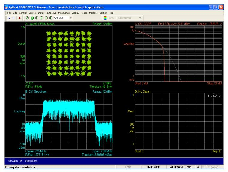
LTE QPSK Tx1 722 MHz, 40W (46 dBm), 10 MHz BW
