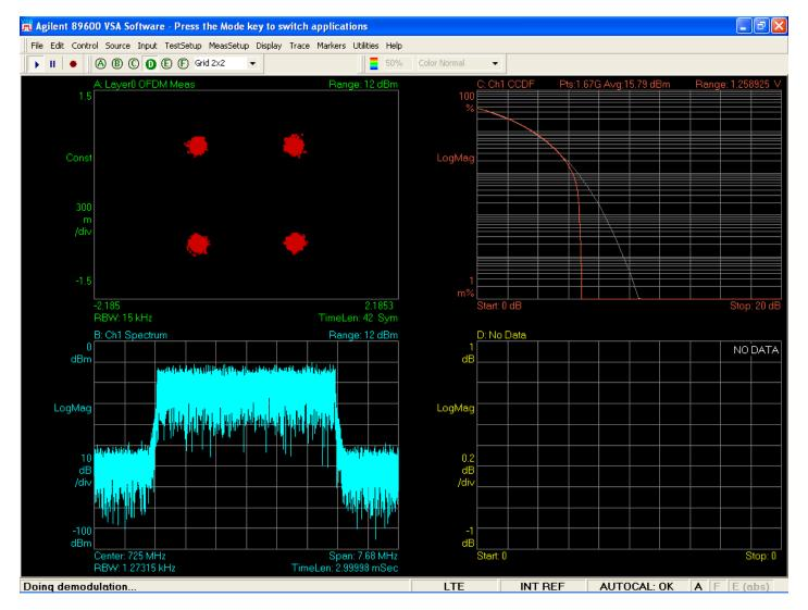
LTE 16QAM Tx1 725 MHz, 40W (46 dBm), 5 MHz BW
