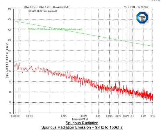
Note: No significant emission (i.e., less than 10dB below the limit) was noted.
