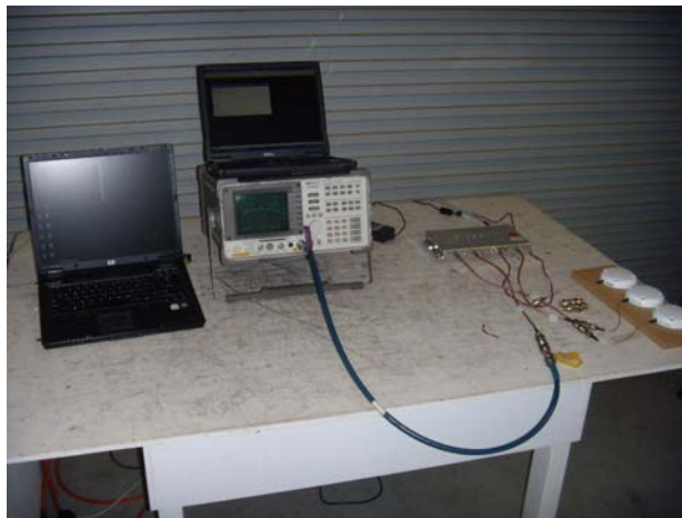
15.247 Antenna Port Conducted Measurement
