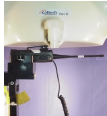
Body-worn SAR Test Setup with Speaker-Microphone & 1.4cm Belt-Clip
