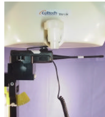
Body-worn SAR Test Setup with 1.4cm Belt-Clip
