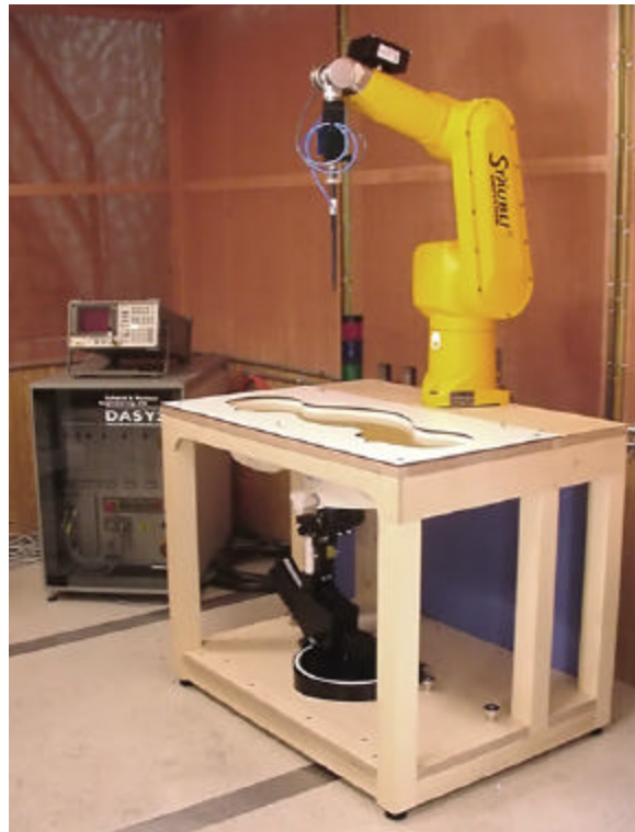
DASY3 SAR Measurement System with SAM phantom
