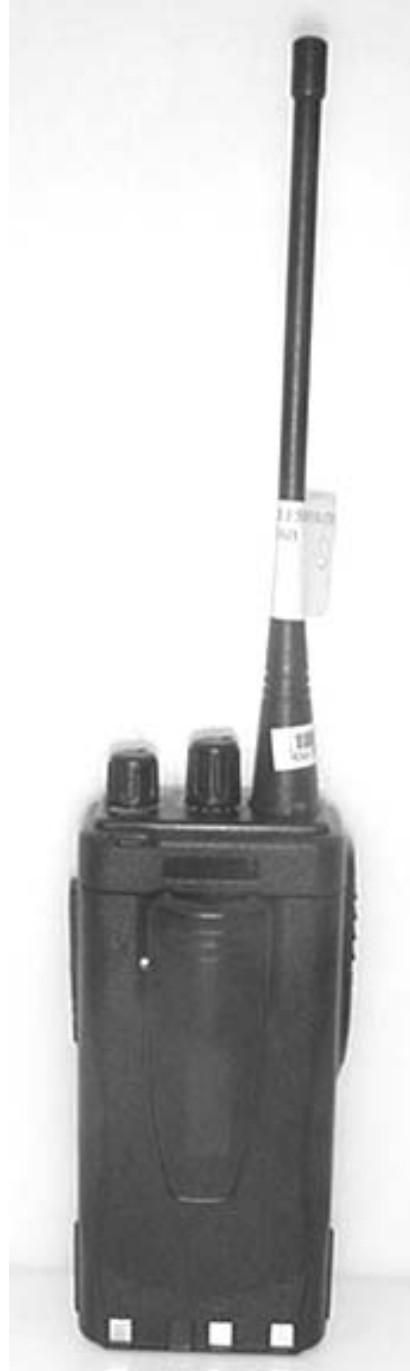
Back of DUT with Belt-Clip
