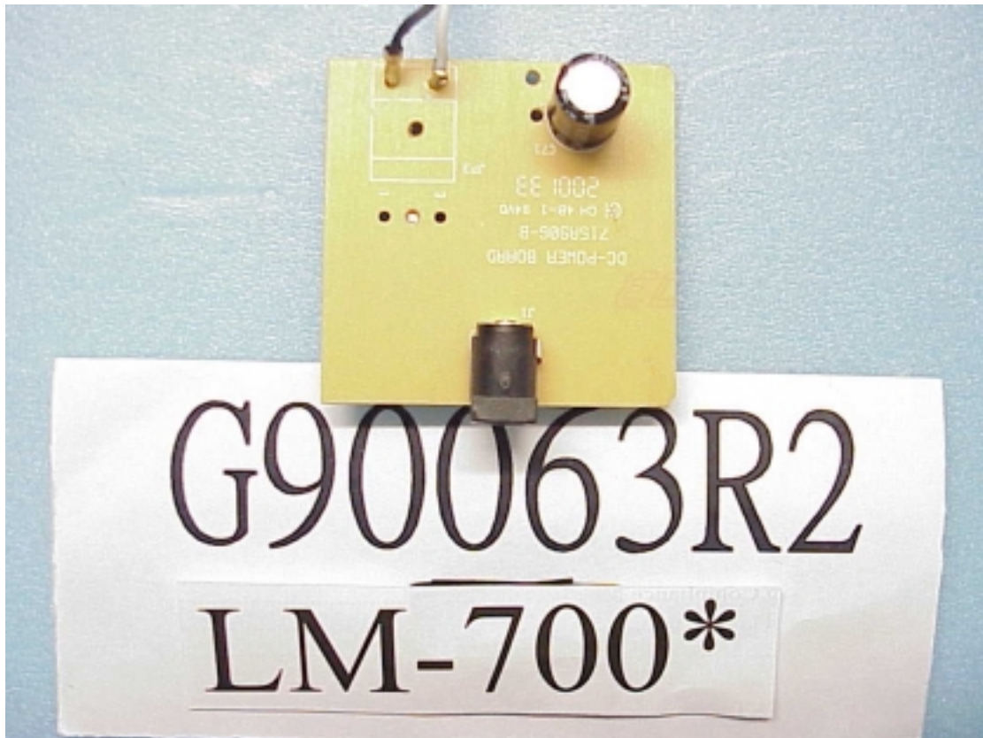
Figure 53 DC Power Board (Component Side), M/N LM-700*
