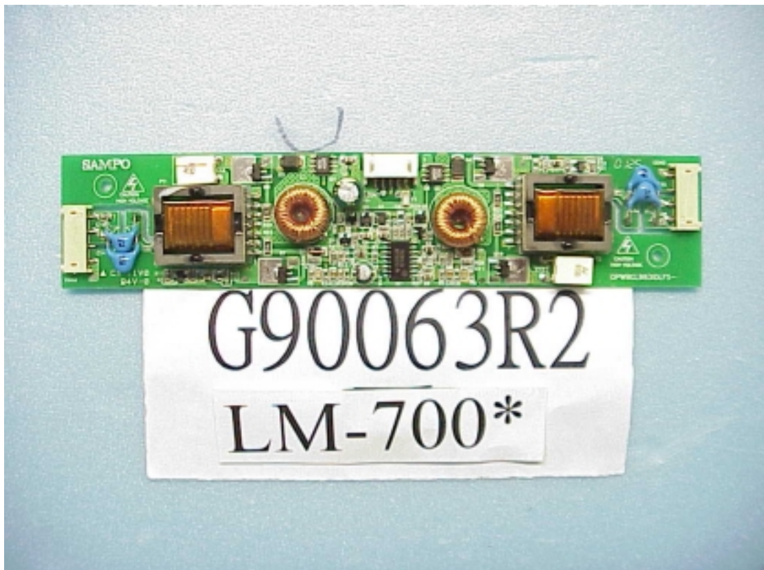
Figure 62 Inverter Board (Component Side), M/N LM-700*
