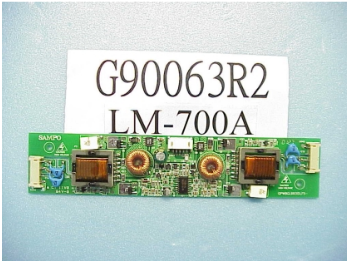
Figure 39 Inverter Board (Component Side), M/N LM-700A
