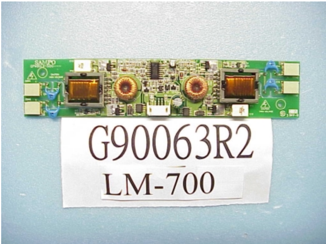
Figure 10 Inverter Board (Component Side), M/N LM-700
