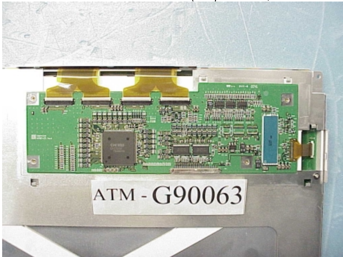
Control Board (Component Side, # 1 Chi Mei LCD Panel)
