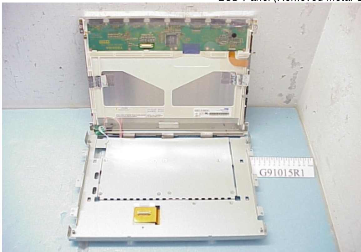
Figure 14 15" LCD Monitor LCD Panel (Removed Metal Cover)
