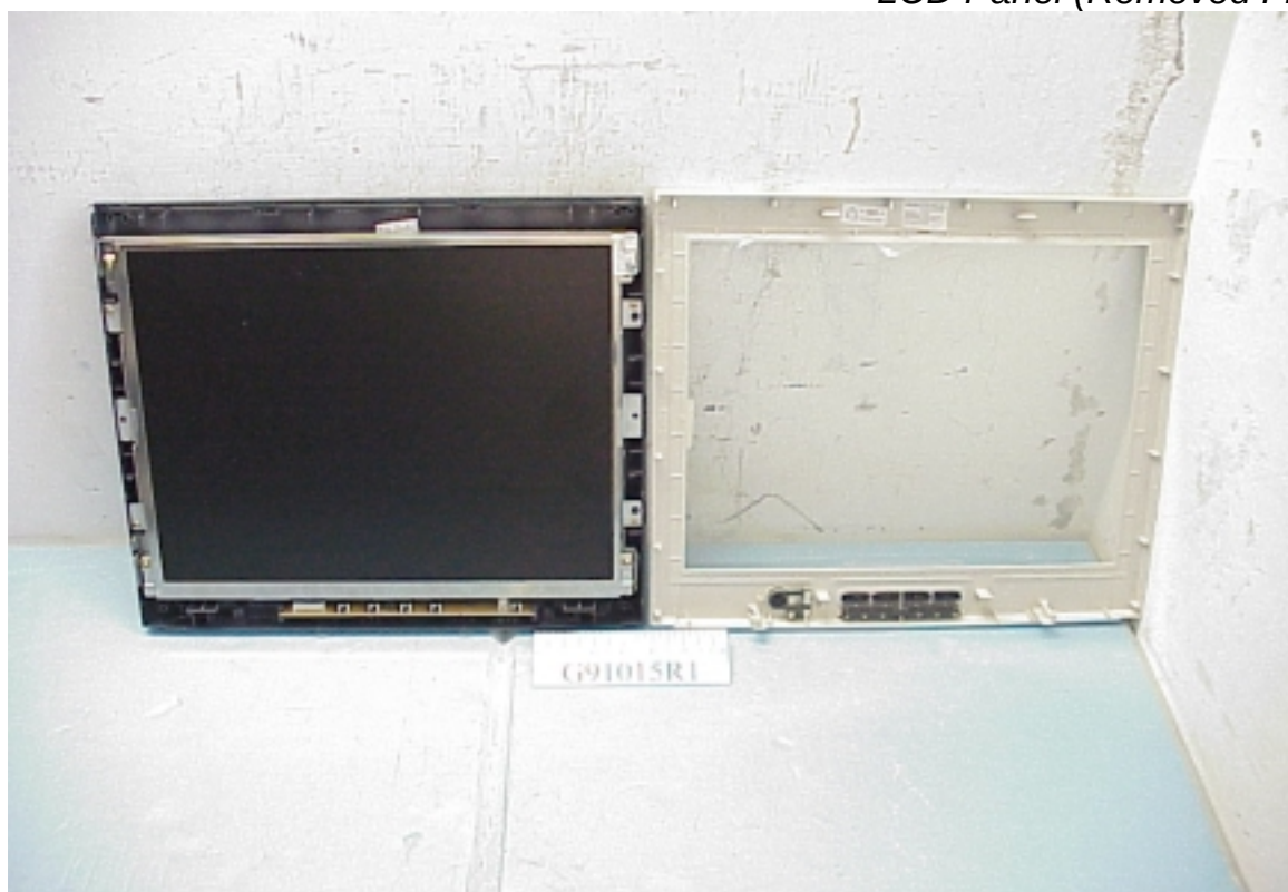
Figure 12 15" LCD Monitor LCD Panel (Removed Frame)
