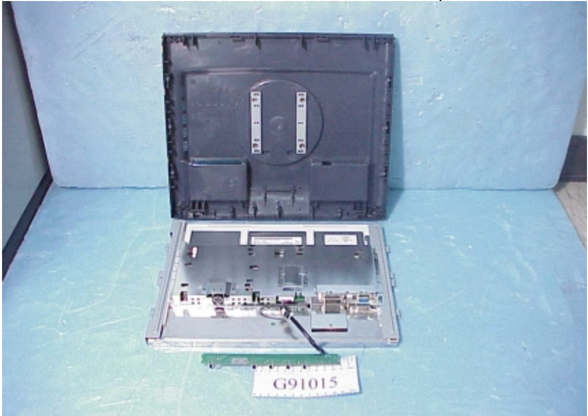
Figure 23 Frame of Internal (Removed Back Cover)
