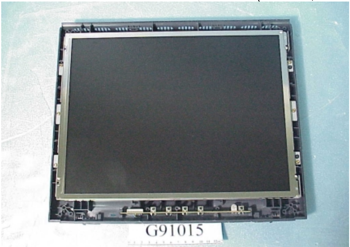
Figure 20 Frame of Internal (LCD Panel, Front Side)
