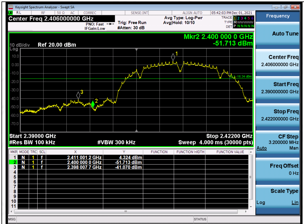
Test_Graph_802.11b_ANT1_2412_1Mbps_Lower Band Edge Emissions
