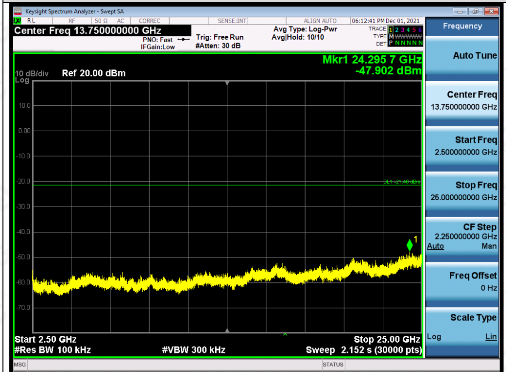
Test_Graph_802.11n20_ANT1_2462_MCS0_Higher Band Emissions
