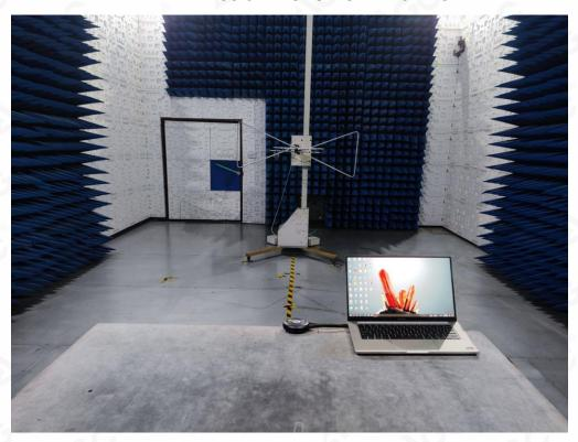
RADIATED EMISSION TEST SETUP ABOVE 1GHz
