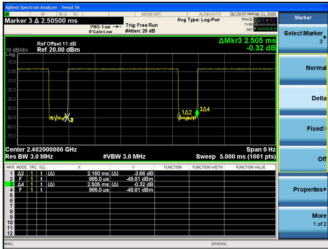
Bluetooth V5.0: Duty cycle factor =  $20\log(\text{duty cycle}) = -4.696\text{dB}$
