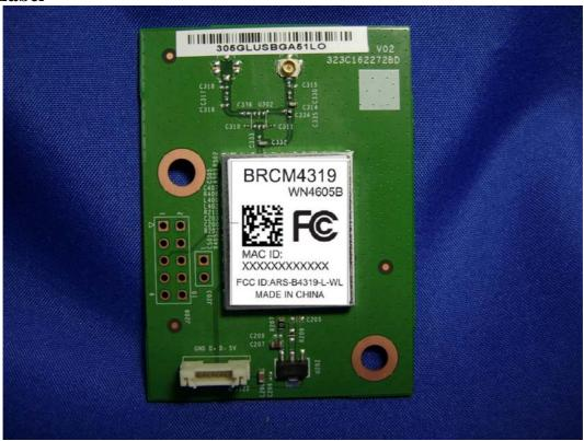
The FCC ID Label and DoC will be placed on the equipment as shown in the photograph below.
