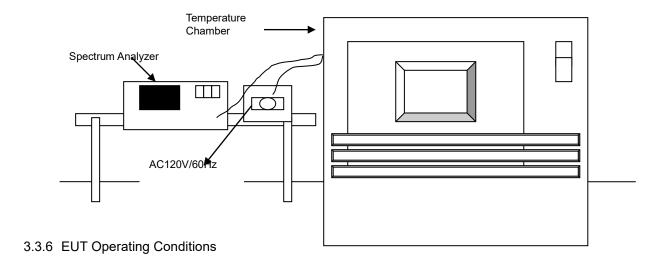
Set the EUT under transmission condition continuously at specific channel frequency.
