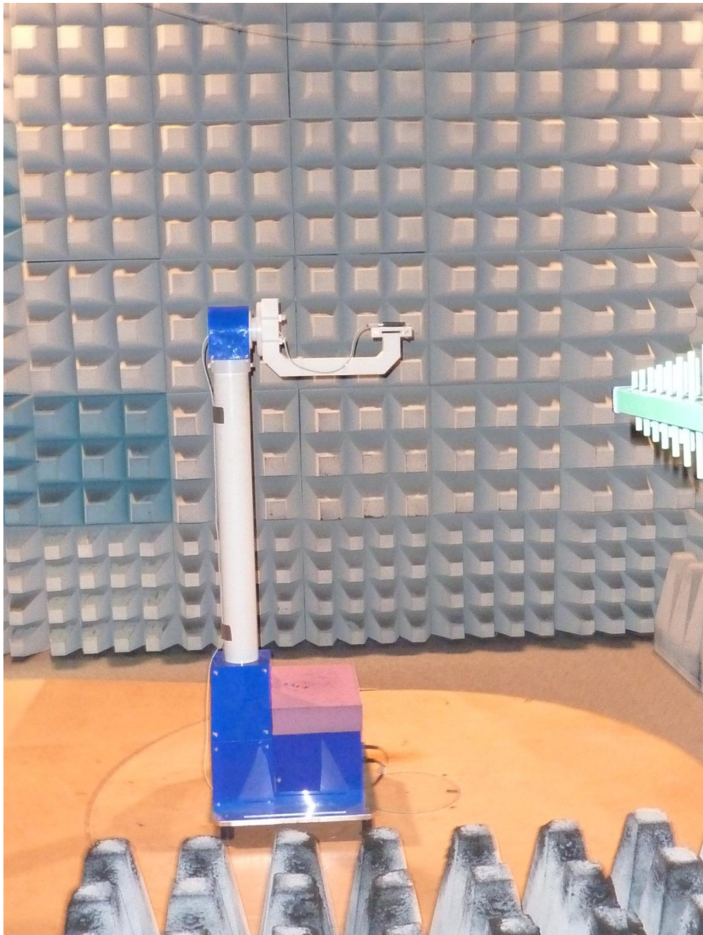
180803_4.JPG: W-LINK STICK, test setup fully anechoic chamber
