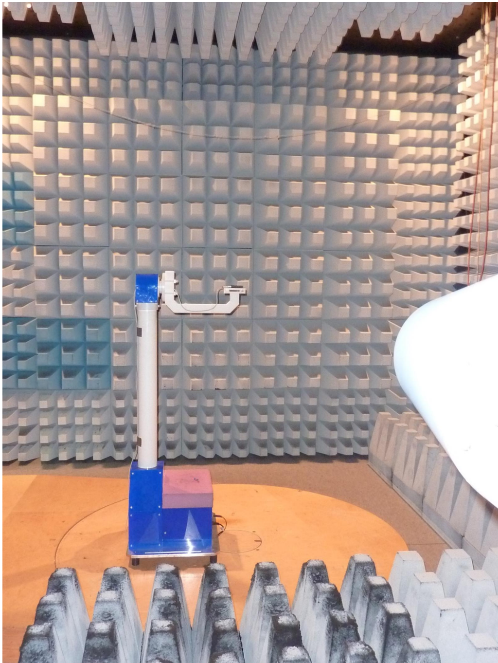
180803_5.JPG: W-LINK STICK, test setup fully anechoic chamber
