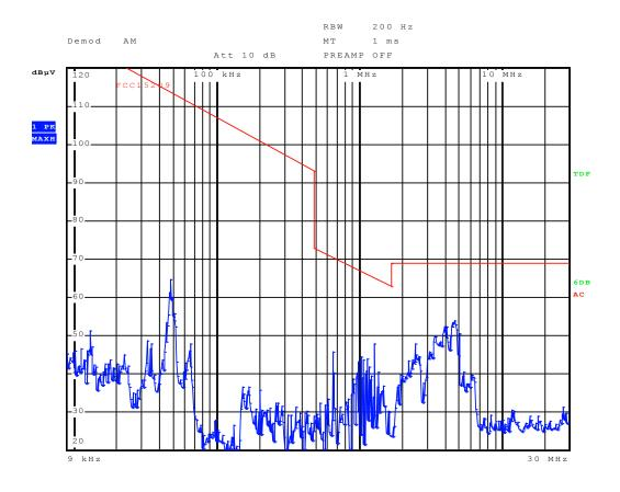
No unwanted emissions in the frequency range 9 kHz - 30 MHz were detected during the exploratory and compliance measurements in either transmit or receive mode. The emissions on other frequencies than 457 kHz are not originating from the Element Barryvox A10012-10000.
