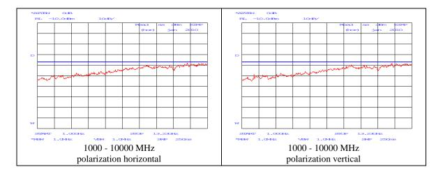
Note: No unwanted emissions with frequencies higher than 1 GHz were found when in receive mode.
