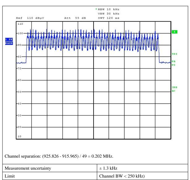
Note: The picture shows that 50 discrete hop frequencies are used. The lowest hop frequency is 915.965 MHz and the highest hop frequency is 925.826 MHz.
