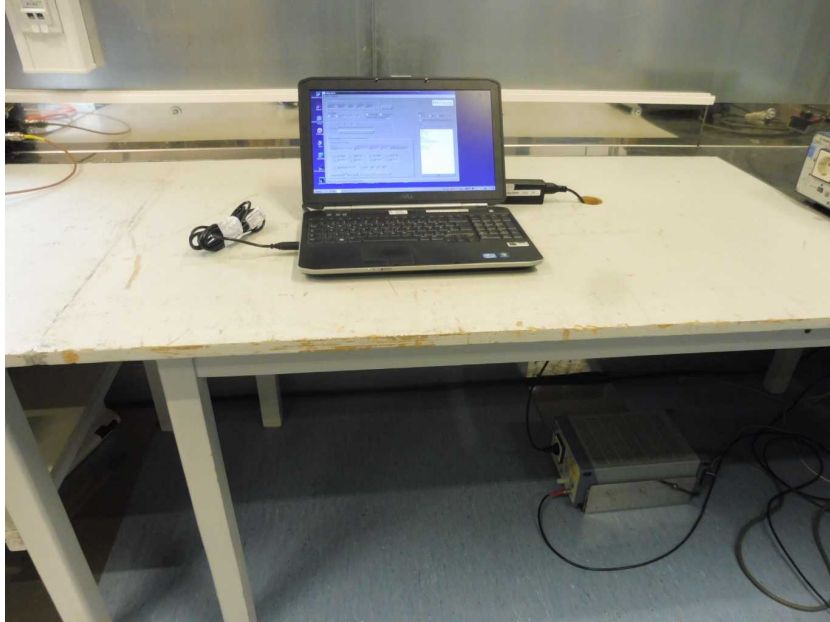
Photo 9: AC conducted emission test setup
