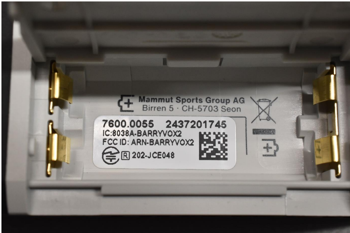
Figure 2 - FCC ID, ISED ID and Giteki mark in the Barryvox 2 battery compartment
