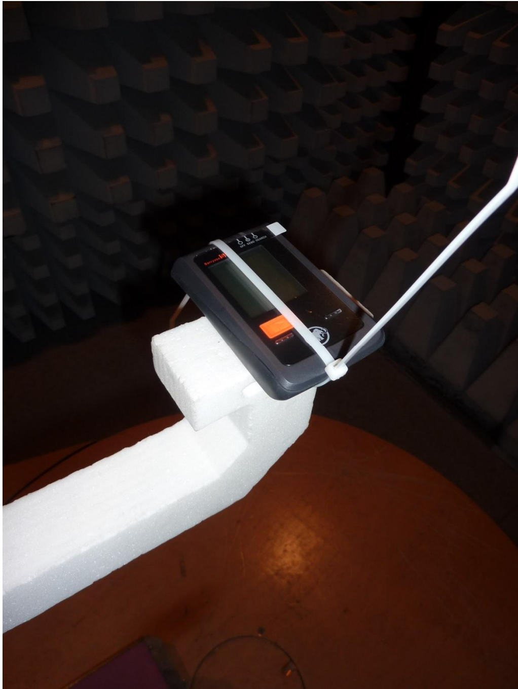
171626_c.JPG: Barryvox S, test setup fully anechoic chamber
