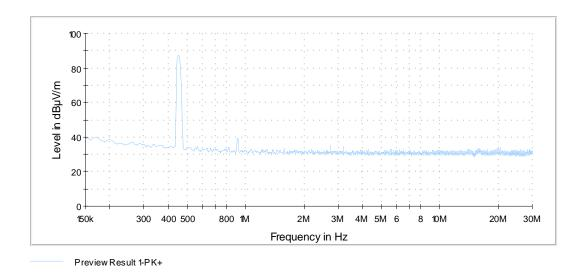
The emissions found in this frequency range are caused by the 457 kHz transceiver of the EUT, which is will be certified under an other FCC 47 CFR Part 15 section. The measurement results for this rule section are documented under PHOENIX TESTLAB GmbH test report reference F17626E2.
