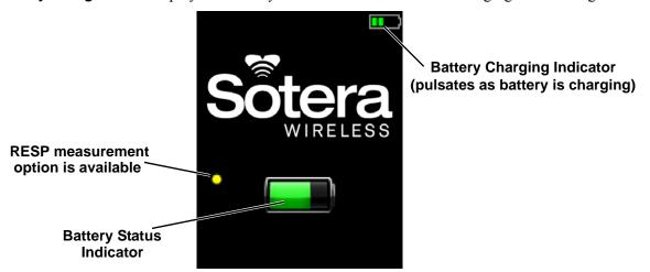
Note: When the yellow dot is displayed on the screen, it indicates the Monitor will measure RESP when a Chest Sensor is connected to a patient. RESP is not available as part of the default set of vital sign measurements and must be purchased separately.
