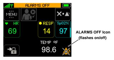
Note: Alerts that indicate the Monitor is unable to measure a vital sign (such as ECG Lead Fail) can not be turned off.
