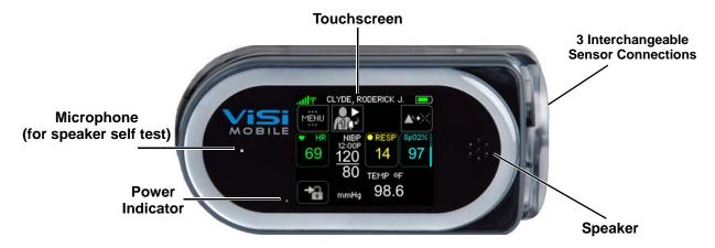
Note: The power indicator shows the level of Monitor's battery charge by flashing green (the battery has at least 2 hours of monitoring time left), yellow (the battery is low with less than 2 hours of monitoring time left), and red (the battery is critically low with less than 30 minutes of monitoring time left).
