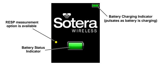
Note: When the yellow dot is displayed on the screen, it indicates the Monitor will measure RESP when a Chest Sensor is connected to a patient. RESP is not available as part of the default set of vital sign measurements and must be purchased separately.
