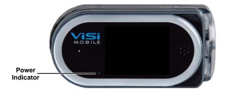
The power indicator will blink while the Monitor is charging: green indicates there is enough charge to monitor a patient for at least two hours; yellow indicates the battery charge is low (less than two hours of monitoring); and red indicates the battery charge is critically low (less than 30 minutes of monitoring).
