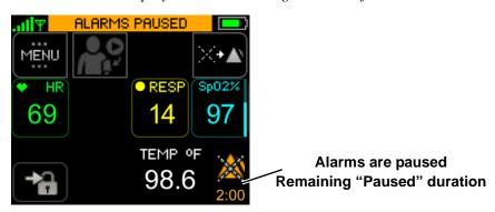
Note: When the clinician logs out of the ViSi Mobile Monitor, the alarms will automatically be resumed.
