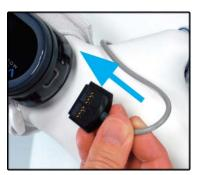
Insert with connector contacts facing upwards
