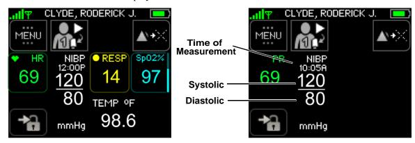
Note: If the NIBP measurement was unsuccessful, the Cuff Module automatically retries to measure the blood pressure. A maximum of 3 attempts will be made. If the failure is due to a cuff leak or cuff occlusion, there is no retry and the LEAK or OCCL message appears on the screen directly below the NIBP label.
