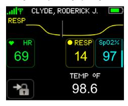
2. To return to the main **Vital Signs** screen, touch the **RESP** numeric. *The RESP waveform is no longer displayed.*
