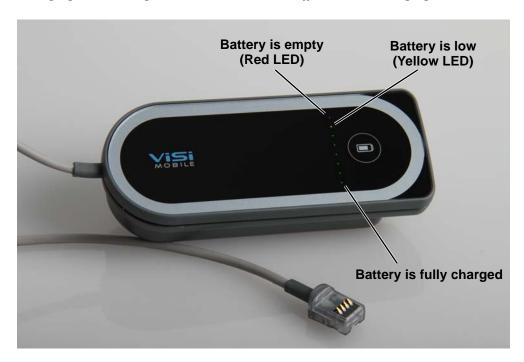
When one of the green charging indicators is flashing, the battery in the Cuff Module is charging. The position of the green charging indicator represents the level of charge. When the charge indicator furthest away from the red charging indicator is flashing, the Cuff Module is fully charged.
