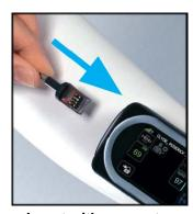
Insert with connectors contacts facing upwards
