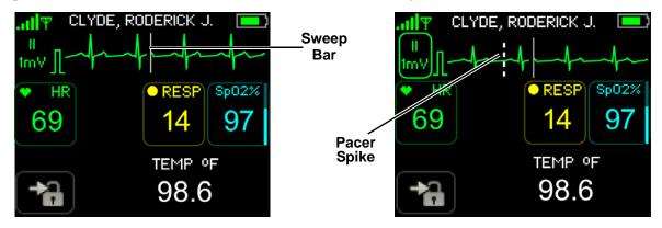
The speed of the waveform display (sweep speed) is scaled to 25 mm/sec for ECG and SpO<sub>2</sub> waveforms.
