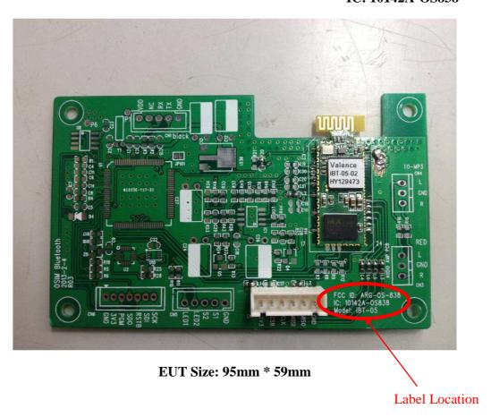
Note: The label would be printed directly on the EUT.
