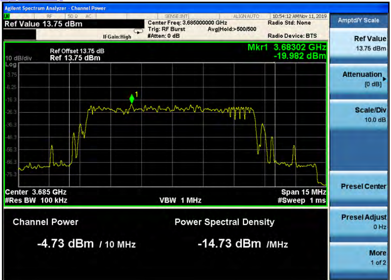
Figure CPE.KDB.7 B: CPE-CBSD EIRP transmit channel power measurement after CPE-CBSD has obtained a grant from test SAS and it is fully utilizing the channel with user data traffic. This plot shows CPE-CBSD obtains connection and can operate at below 23dBm/10MHz EIRP
