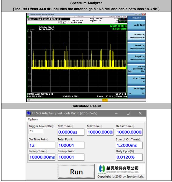
The sum of On Time (aggregated time from marker 1 to 2): 1.2ms < 1s, Pass.
