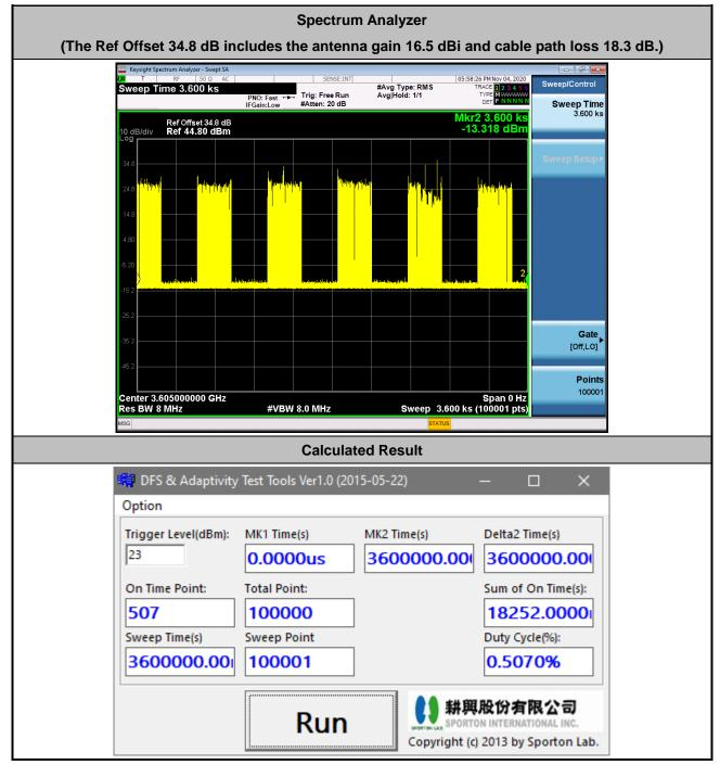
The sum of On Time (aggregated time from marker 1 to 2): 18.25s < 20s, Pass.
