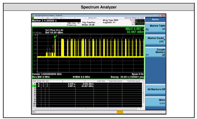
Note: The Ref Offset 34.8 dB includes the antenna gain 16.5 dBi and cable path loss 18.3 dB.
