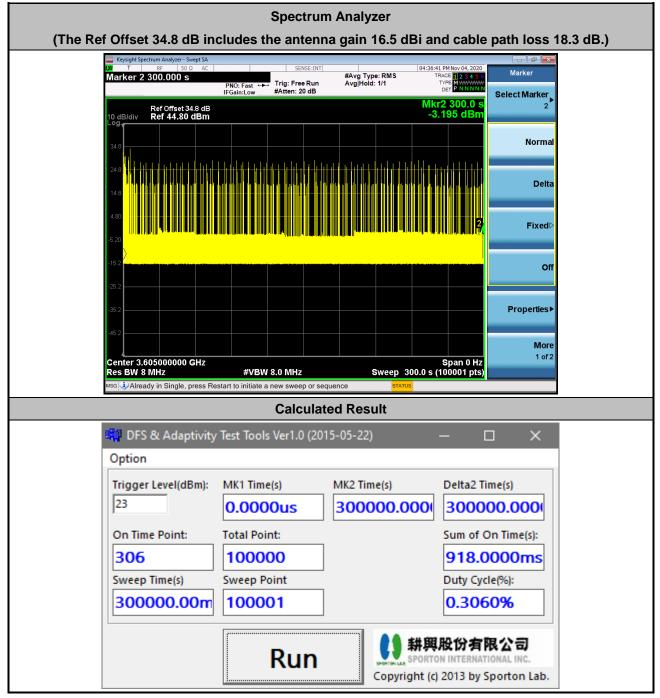
The sum of On Time (aggregated time from marker 1 to 2): 918ms < 10s, Pass.
