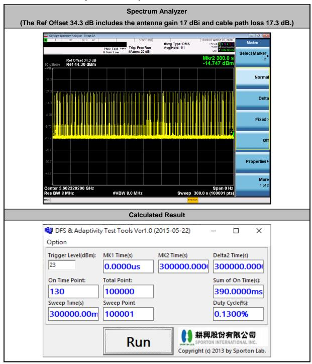
The sum of On Time (aggregated time from marker 1 to 2): 390ms < 10s, Pass.
