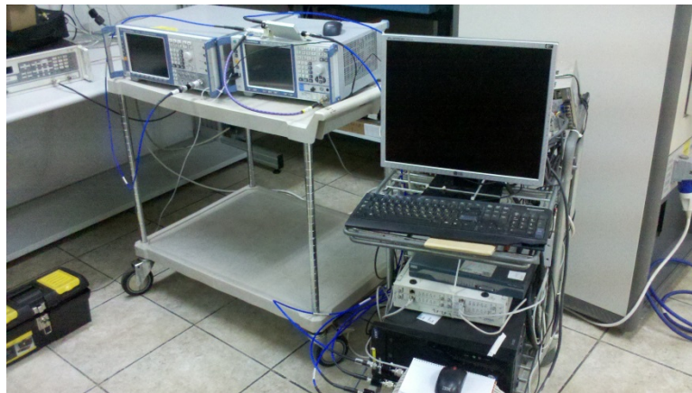
Photograph 8.1.2 Test setup for contention-based protocol verification test
