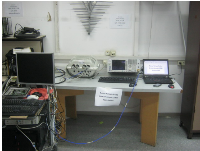
Figure 2. Conducted Emission From Antenna Port Tests
