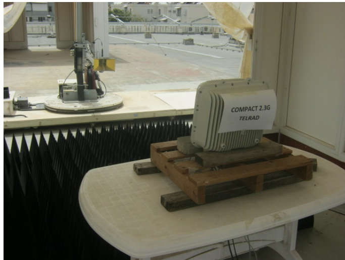
Figure 6. Radiated Emission Test
