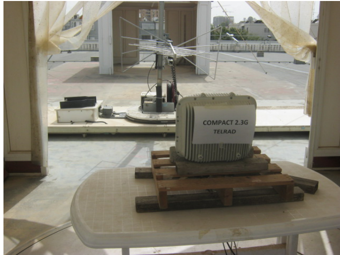
Figure 5. Radiated Emission Test
