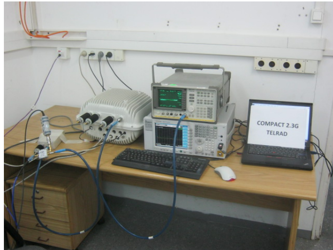
Figure 3. Conducted Emission From Antenna Port Tests
