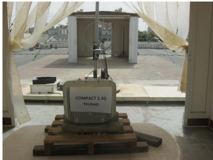
Figure 4. Radiated Emission Test
