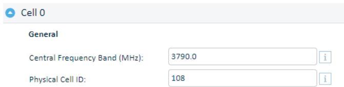
Figure 44: BREEZEVIEW -ENB CELL0 deployment tab when in DualCarrierAggregation
