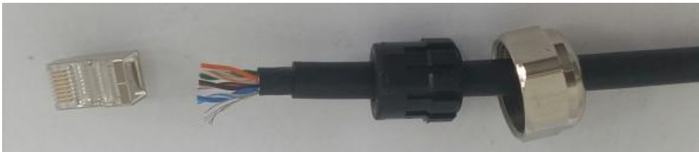
Figure 2-5: Cable preparation for Outdoor Unit
