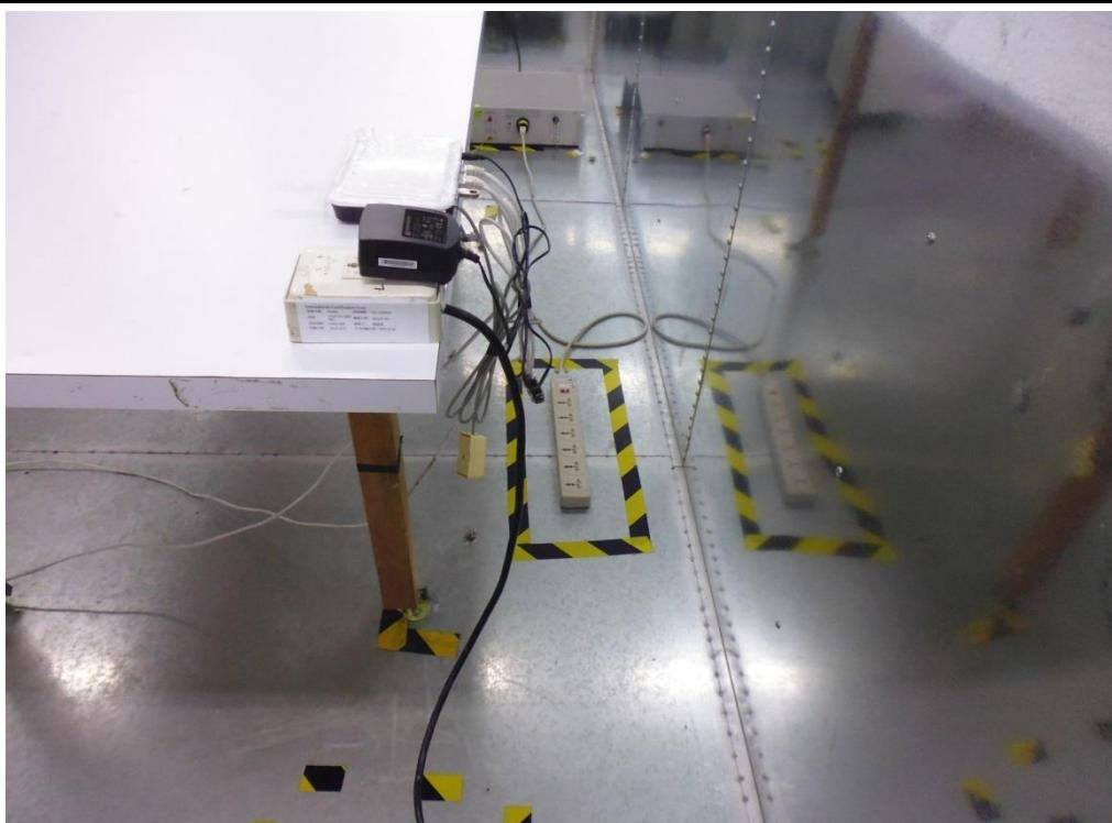
**Radiated Emission Below 1GHz Test**
