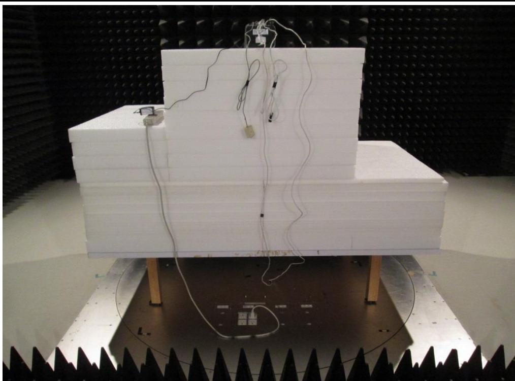
**Radiated Emission Above 1GHz Test**
