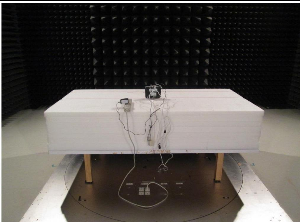
**Radiated Emission Above 1GHz Test**
