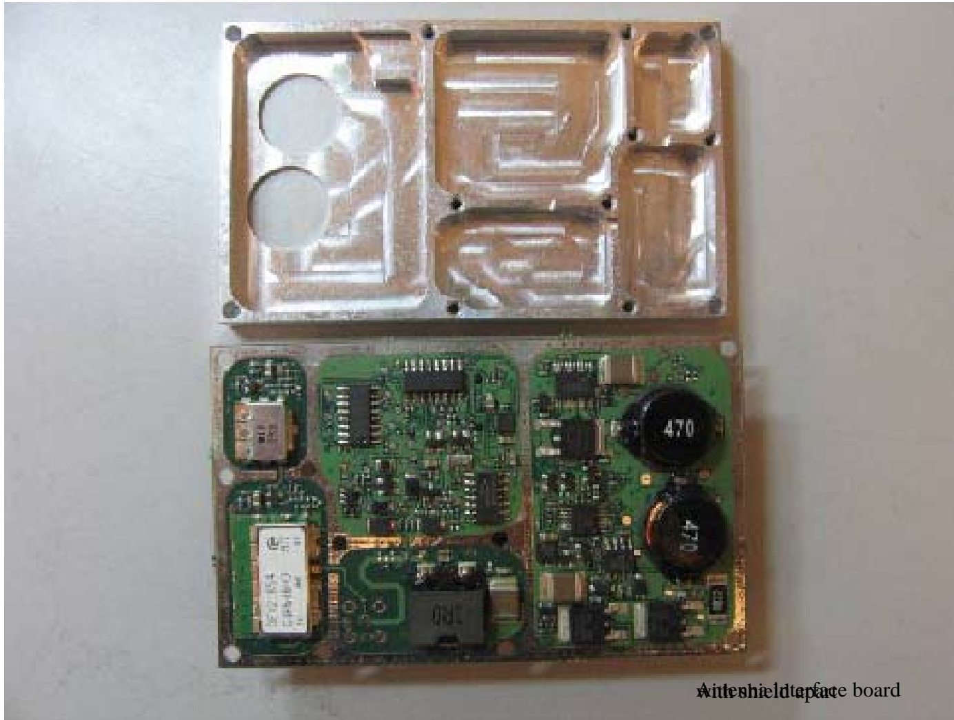
Land Mobile BGAN Terminal, RF-7800B-VU104 Antenna Interface Board Underside – Without Shield. Shield Shown
