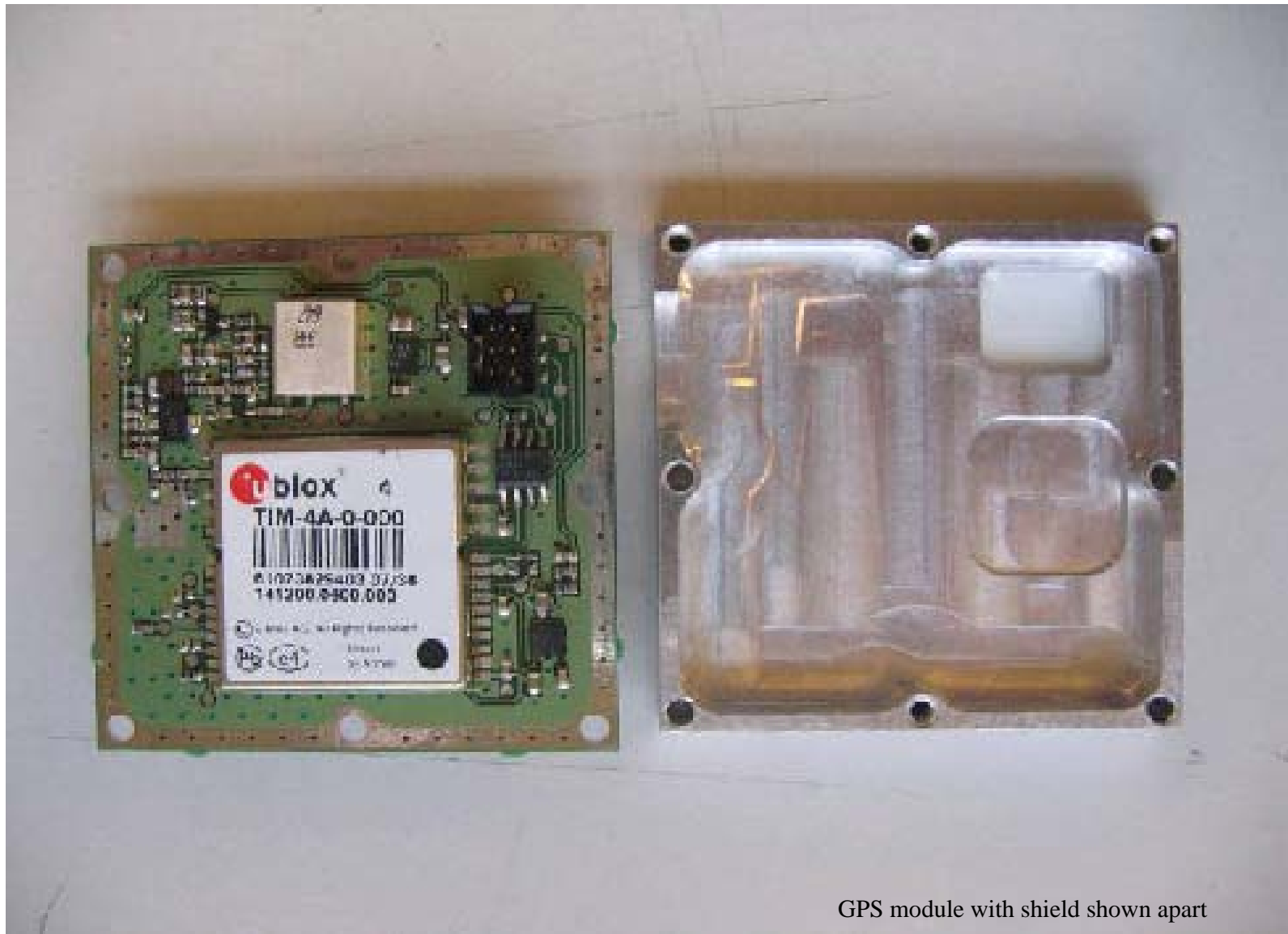
Land Mobile BGAN Terminal, RF-7800B-VU104 GPS Module Underside – Without Shield. Shield Shown
