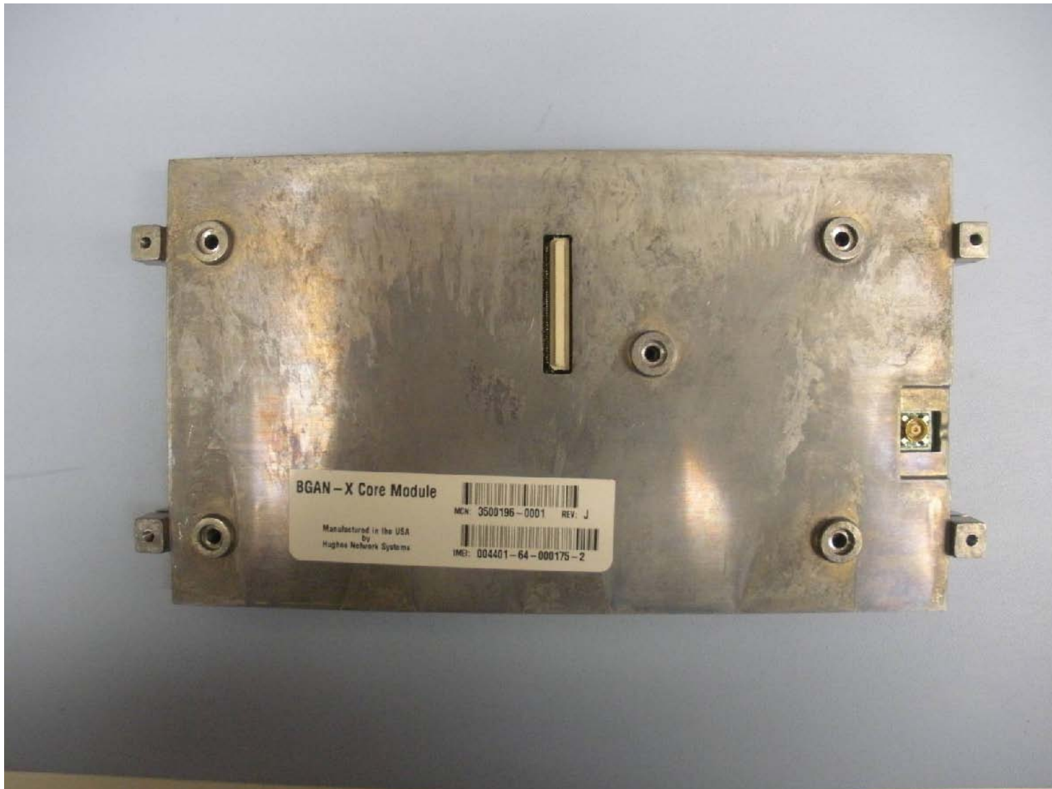
Land Mobile BGAN Terminal, RF-7800B-VU104 Core Module Shield - Underside
