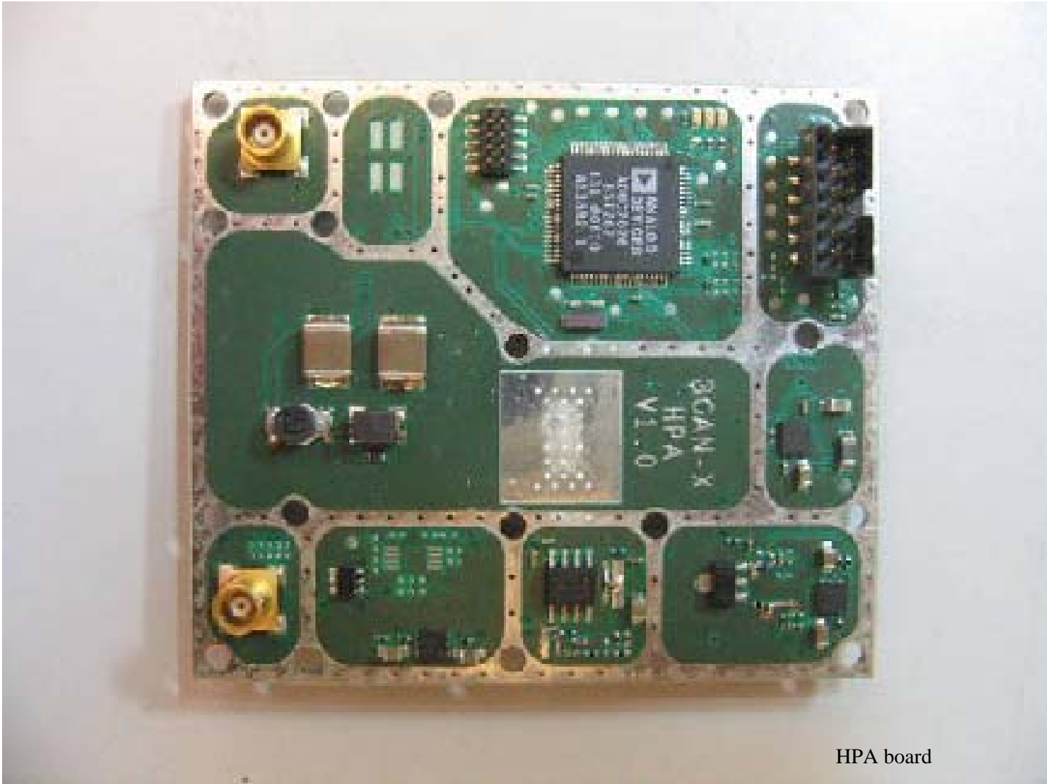
Land Mobile BGAN Terminal, RF-7800B-VU104 HPA Board Topside – Without Shield
