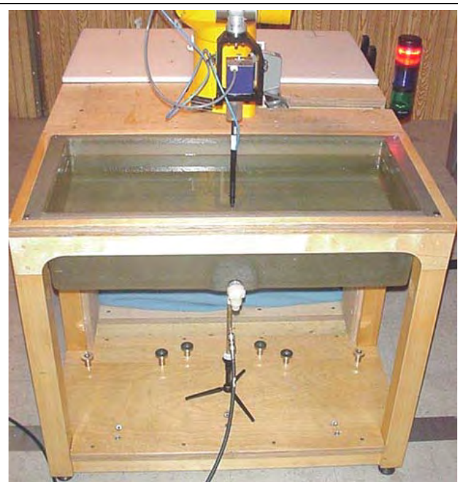
DASY4 SAR System with Baski Fiberglass Planar Phantom
