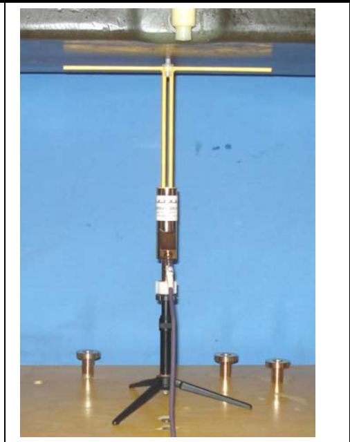
System Performance Check Measurement Setup Diagram (IEEE 1528-2003) 450 MHz SPEAG Validation Dipole Setup
