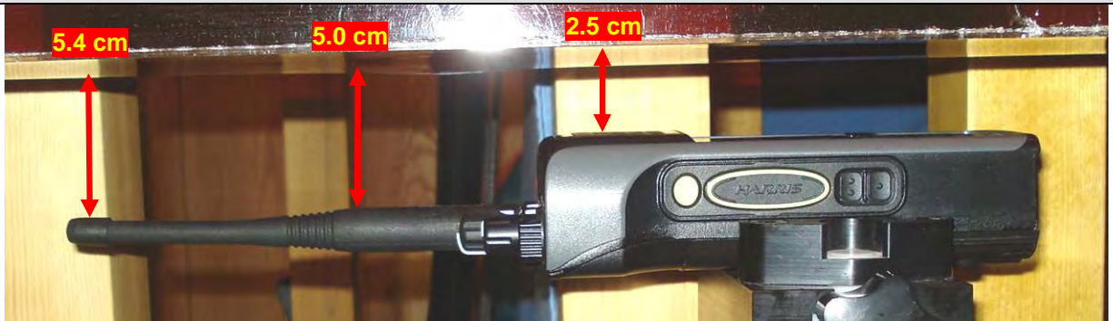
Face-held with Battery e and Antenna #1
