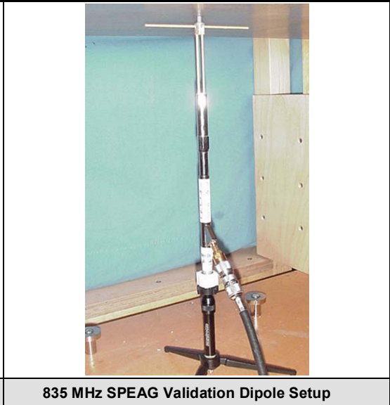
System Performance Check Measurement Setup Diagram (IEEE 1528-2003) 835 MHz SPEAG Validation Dipole Setup
