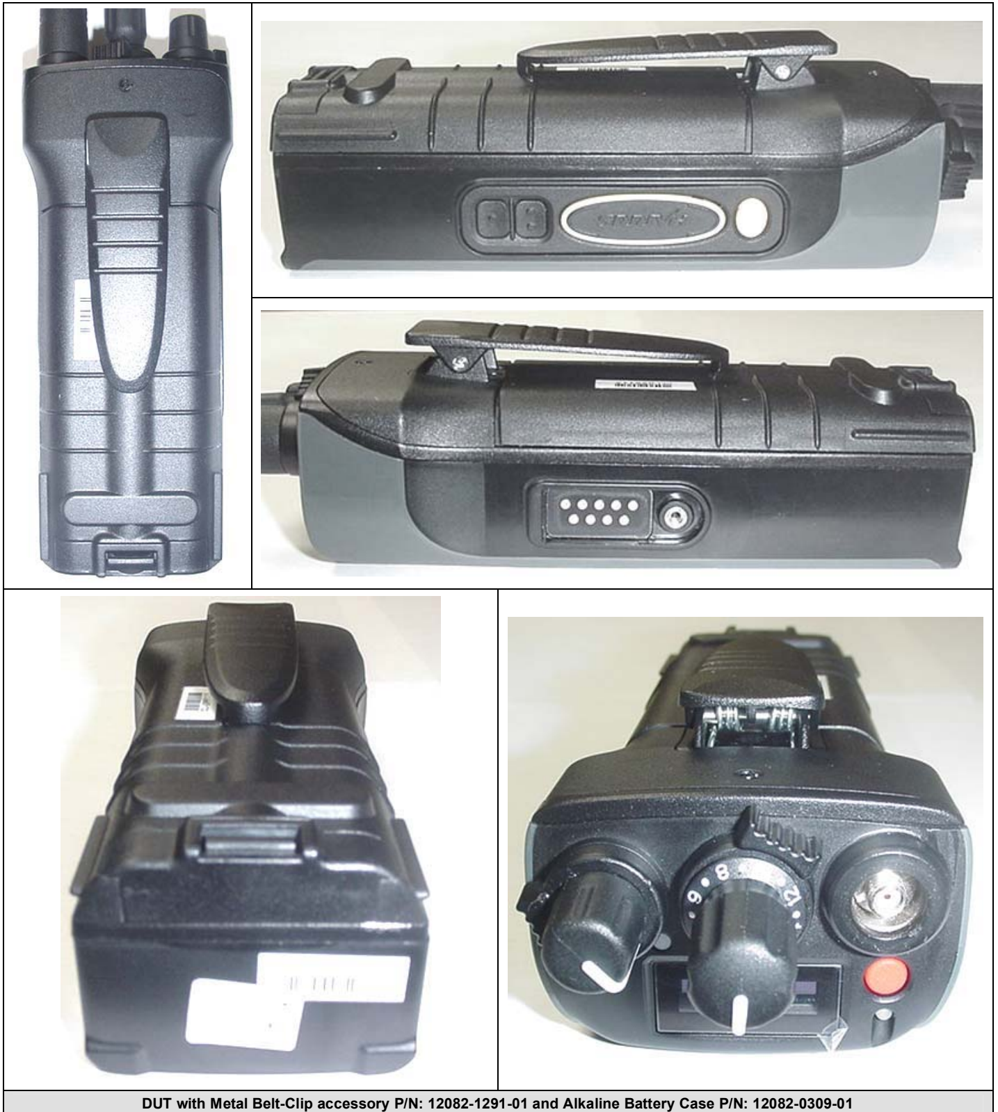
DUT with Metal Belt-Clip accessory P/N: 12082-1291-01 and Alkaline Battery Case P/N: 12082-0309-01
