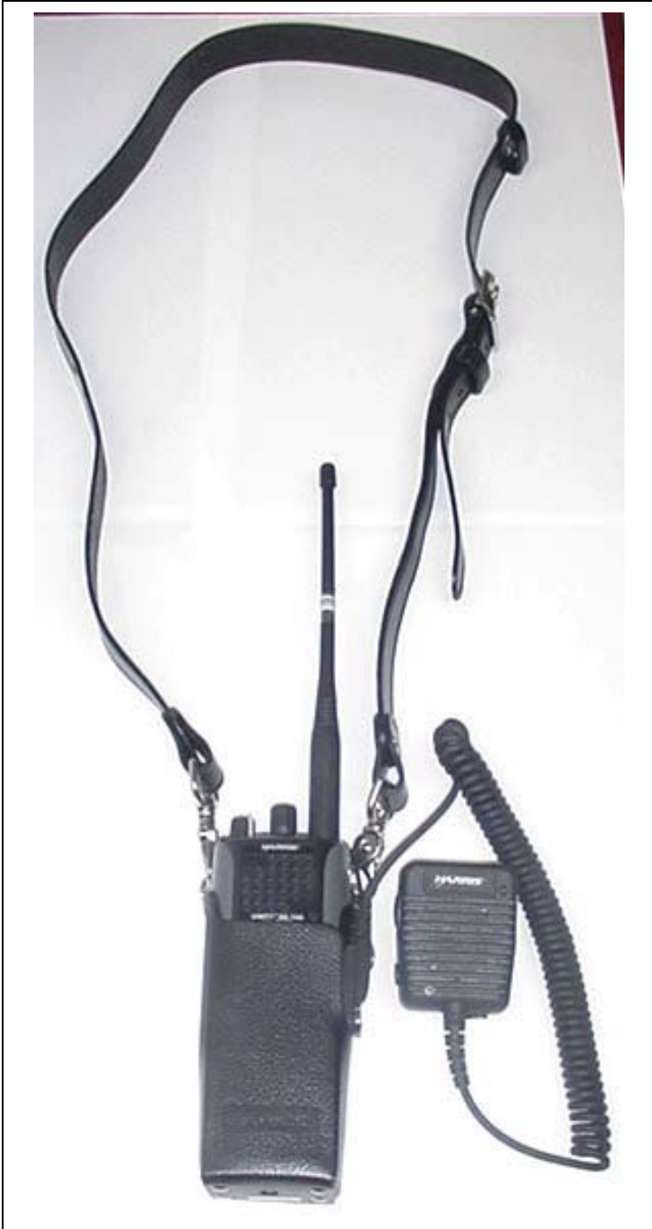
Front of DUT with Leather Case (Full) accessory P/N: 12082-0500-01, Shoulder Strap P/N: 12082-0505-01 & Speaker-Mic P/N: 12082-0600-01
