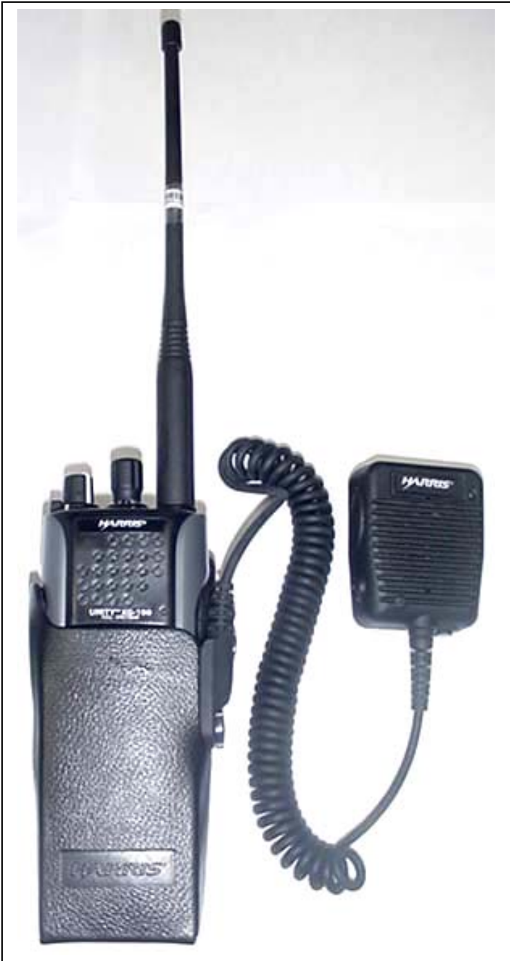
Front of DUT with Leather Case (Full) P/N: 12082-0502-02 and Swivel Belt-Loop (3") accessory & Speaker-Mic P/N: 12082-0600-01
