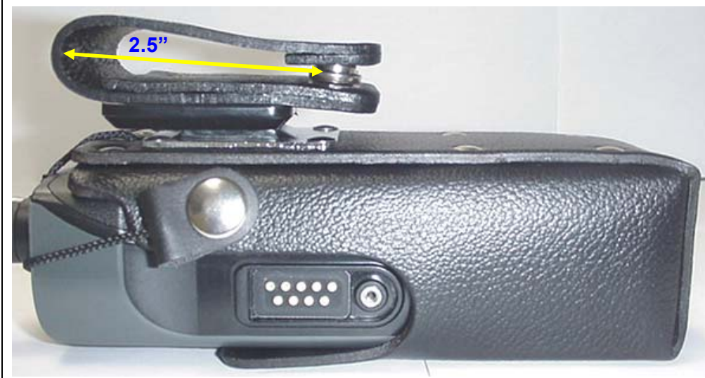
Left & Right sides of DUT with Leather Case (Full) P/N: 12082-0502-01 and Swivel Belt-Loop (2.5")
