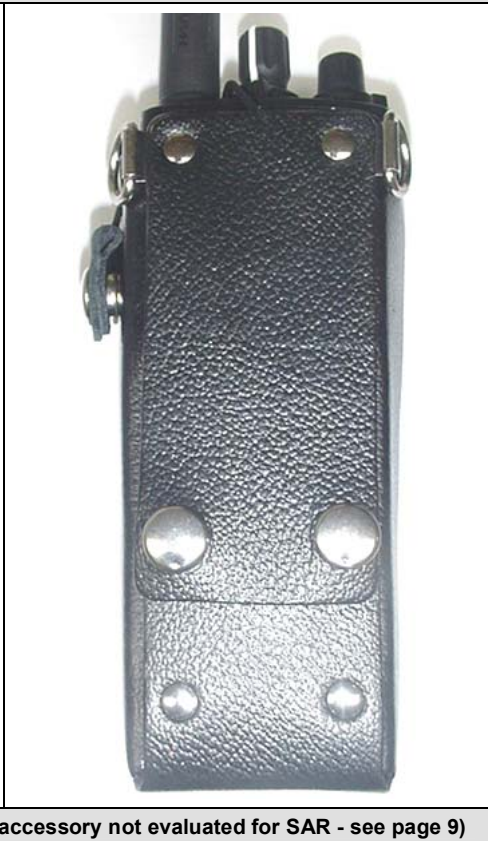
Left & Right sides of DUT with Leather Case (Half) and D-Rings accessory P/N: 12082-0501-01
