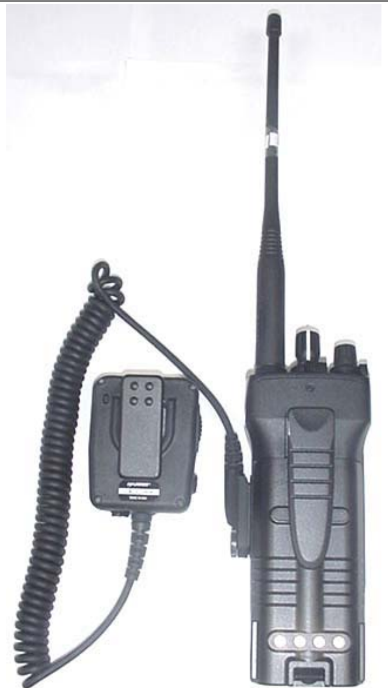
Back of DUT with Metal Belt-Clip accessory P/N: 12082-1291-01 and Speaker-Microphone audio accessory P/N: 12082-0600-01
