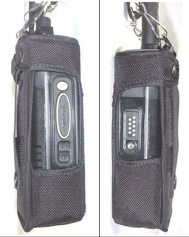
Left & Right Side of DUT with Nylon Case P/N: 12082-0512-01
