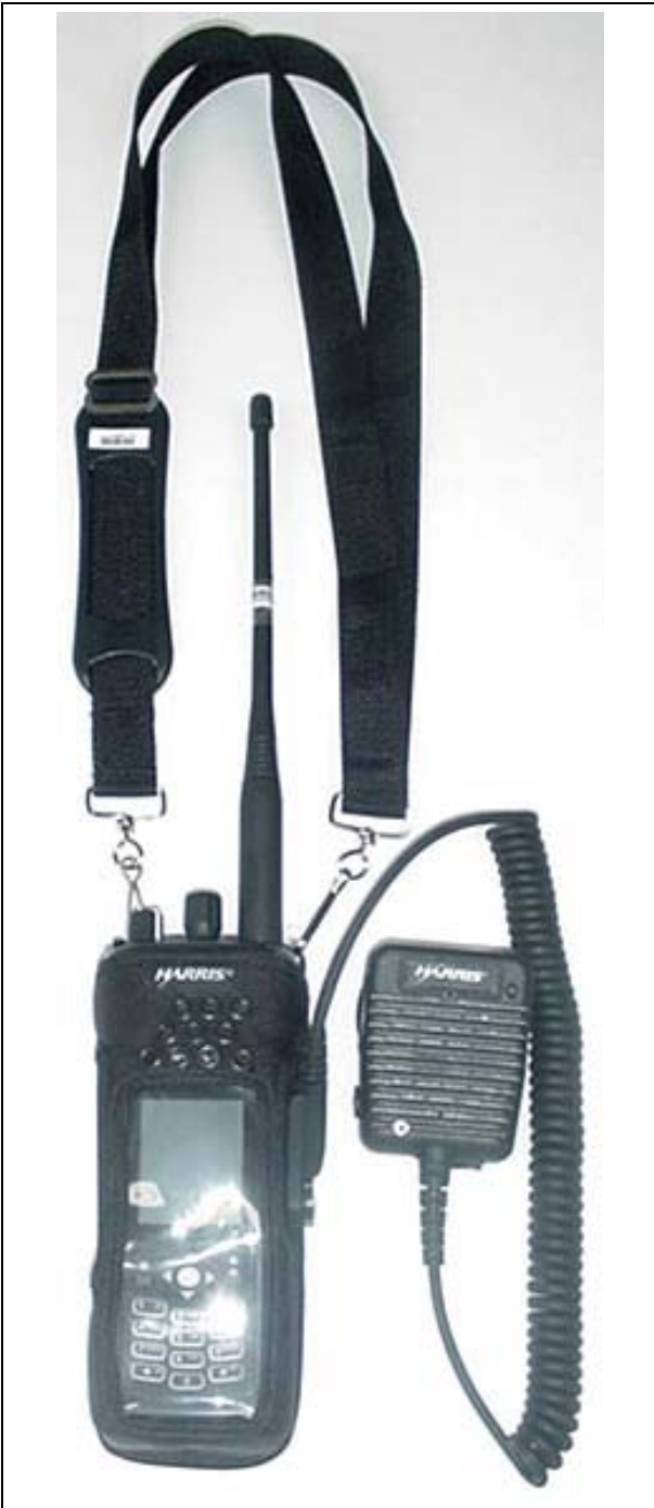
Front of DUT with Nylon Case (Window) accessory P/N: 12082-0512-01, Shoulder Strap P/N: 12082-0504-01 and Speaker-Microphone P/N: 12082-0600-01
