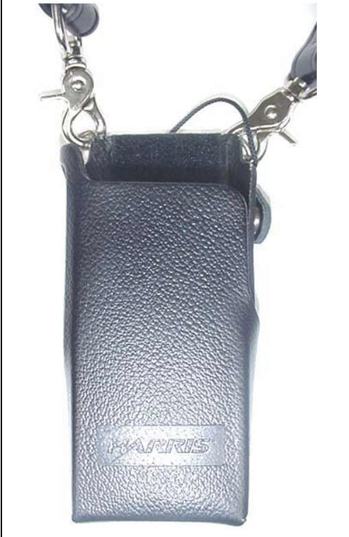
Front & Back of DUT - Leather Case (Full) Metal D-Rings attached to Shoulder Strap Metal Clasps
