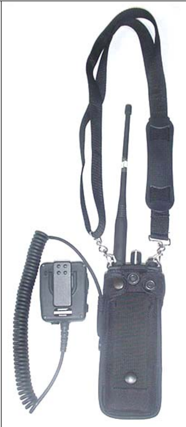
Back of DUT with Nylon Case (Window) accessory P/N: 12082-0512-01, Shoulder Strap P/N: 12082-0504-01 and Speaker-Microphone P/N: 12082-0600-01
