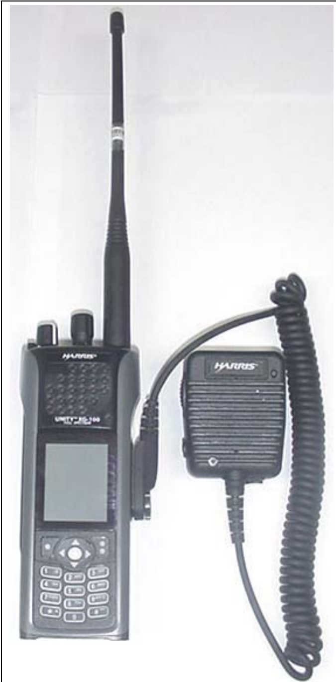
Front of DUT with Metal Belt-Clip accessory P/N: 12082-1291-01 and Speaker-Microphone audio accessory P/N: 12082-0600-01
