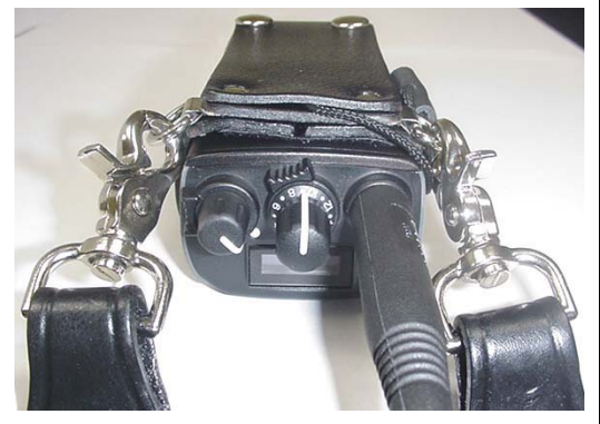
Bottom end of DUT w/ Leather Case P/N: 12082-0500-01 & Shoulder Strap P/N: 12082-0505-01
