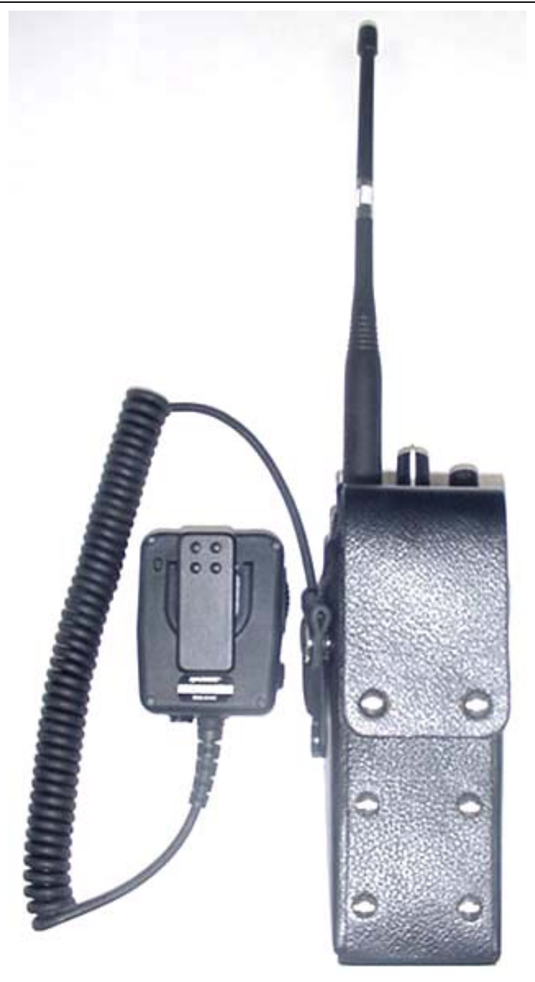
Back of DUT with Leather Case (Full) P/N: 12082-0502-02 and Swivel Belt-Loop (3") accessory & Speaker-Mic P/N: 12082-0600-01
