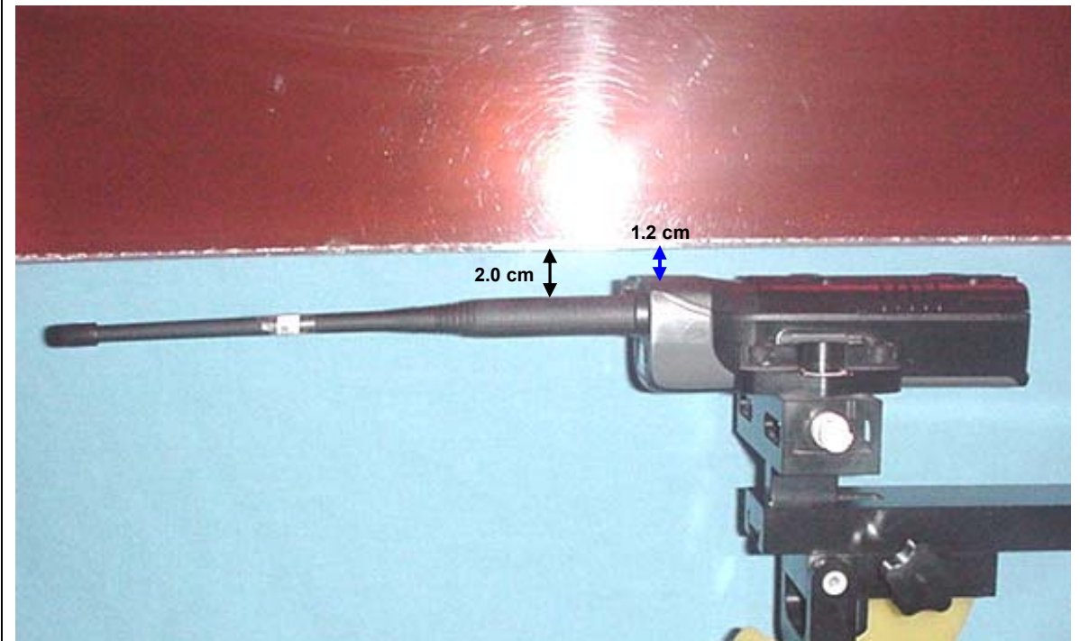
Back side of DUT without body-worn & audio accessories (“Baseline” Highest SAR Battery Search)
