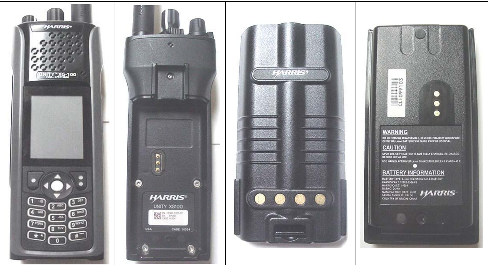
Front of DUT Back of DUT w/ battery removed Lithium-ion Battery P/N: 12082-0308-01 Lithium-ion Battery P/N: 12082-0308-01
