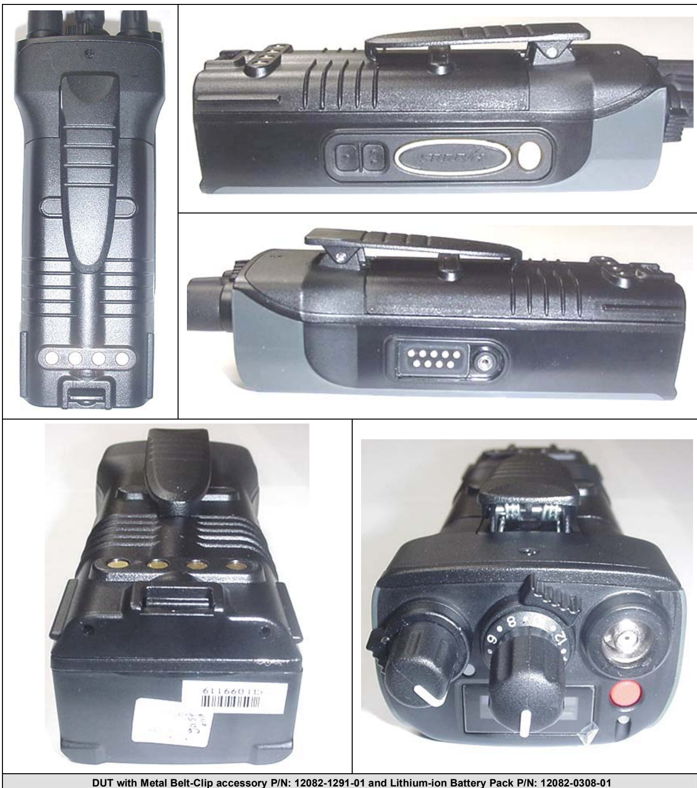
DUT with Metal Belt-Clip accessory P/N: 12082-1291-01 and Lithium-ion Battery Pack P/N: 12082-0308-01
