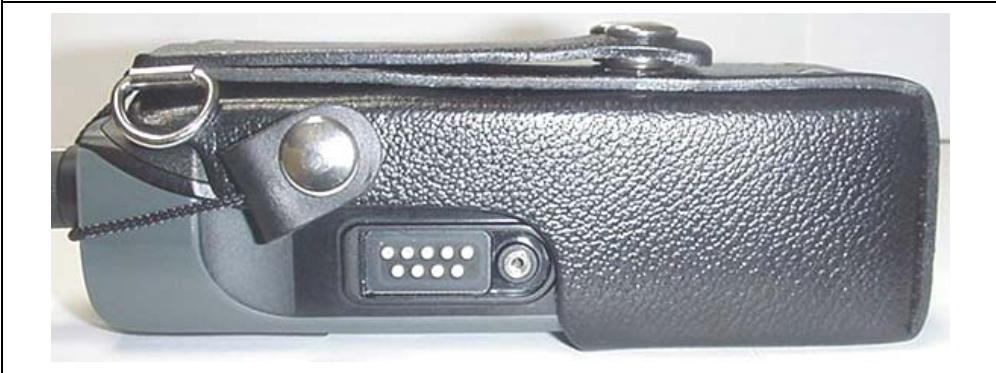
Left & Right sides of DUT with Leather Case (Half) and D-Rings accessory P/N: 12082-0501-01
