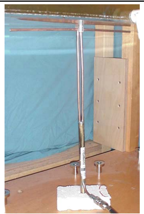
300 MHz Validation Dipole Setup
