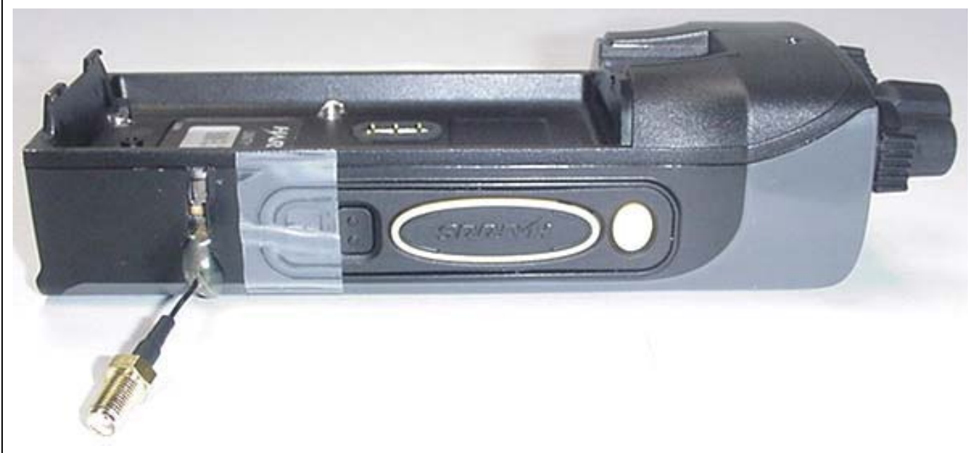
DUT with RF Connector for Bluetooth Conducted Output Power Measurements (modified after Bluetooth SAR evaluations completed)
