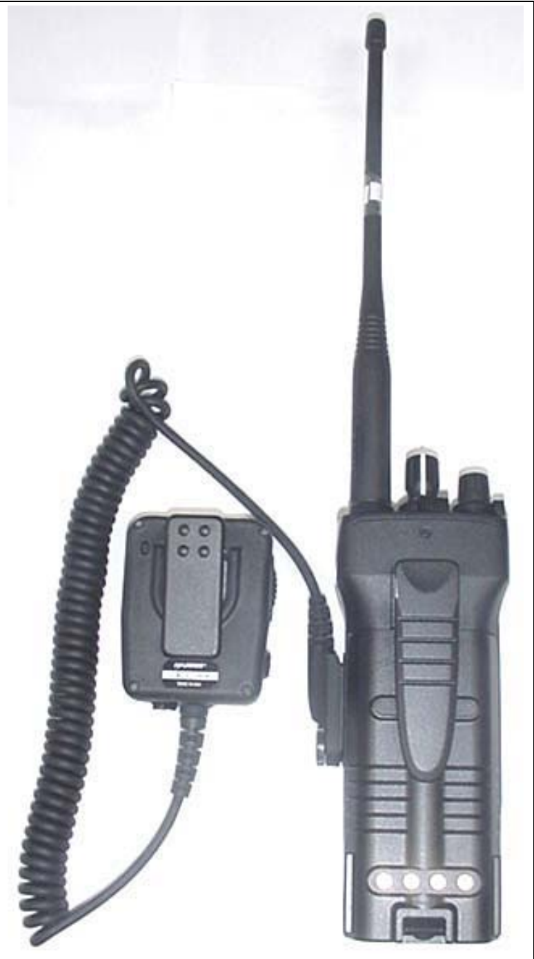
Back of DUT with Metal Belt-Clip accessory P/N: 12082-1291-01 and Speaker-Microphone audio accessory P/N: 12082-0600-01
