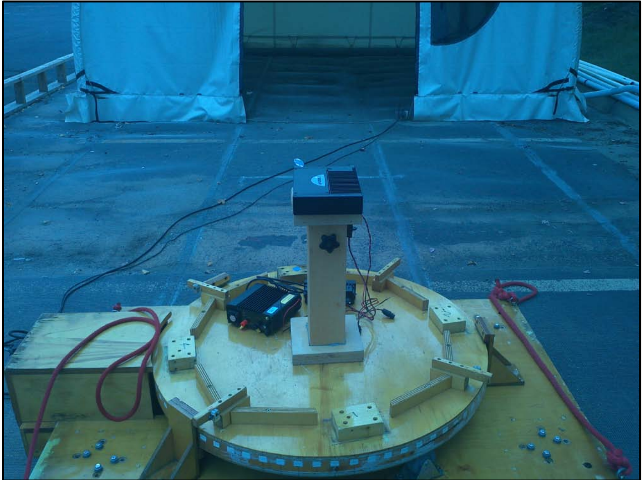
Photograph 1: Radiated Emissions (Spurious/Harmonics) – Front View
